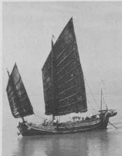
Fishing junks, although seagoing, are usually smaller than the trading types, and range up to 90' over all. They perform the functions of trawlers, purse seiners, and line-fishermen.
