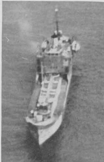
Two versions of small tankers with "economy" hull designs have been observed in quantity, both closely similar to the Type "E (Modified)" cargo carrier in dimensions and general design features. Although no statistics are available, tonnage is believed to approximate closely that of the "E (Modified)" vessels. Note that the trunked-deck version, which probably has a slightly larger barrel capacity, burns coal while the other small-stack design is probably Diesel-powered.
