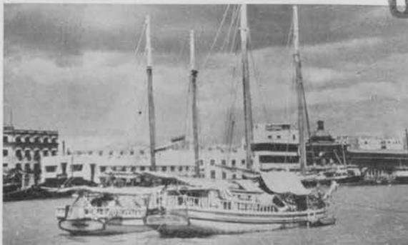
◀ There are well over 200 sailing vessels registered in the P. I., most of which engage in inter-island trade or fishing. The majority of these run from 10 to 40 tons, although a few range up to 70' long and 100 gross tons. Their appearance is fairly standard with two masts forward, deckhouse aft. ▶
