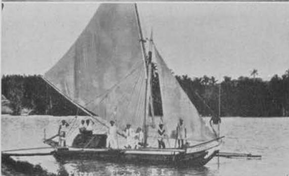
◀ The BATEL is a 40' to 50', 20 to 40 ton dugout or plank-built craft fitted with sails and outriggers. These carry on a great deal of the inter-island native passenger and utility functions. ▶
