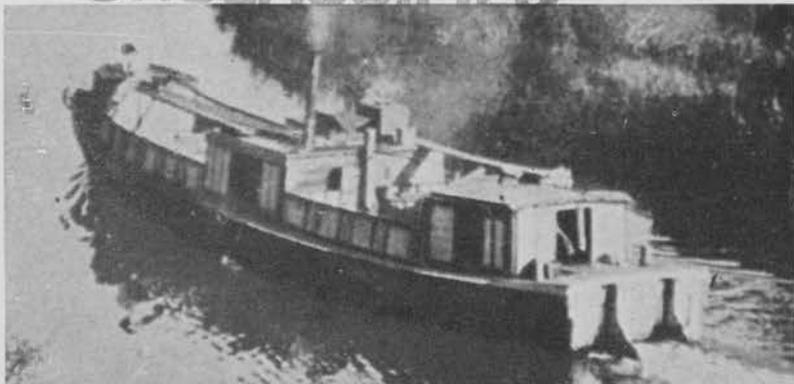
Most cargo barges are nonpowered, and rely mainly on towboats for all transport. However, during the war a great many of them have undoubtedly been fitted with machinery, such as the one above, or with sails for coastal transport. The aerial photo at right shows a group of non-propelled barges beached at Paramushiro.
