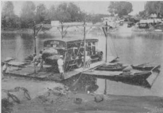
▲ Another cable-drawn type is this fully loaded, native-built pontoon for ferrying across the Labo River, Philippines. None of these ferries appear to employ the automobile's motive power as a means of propulsion.
