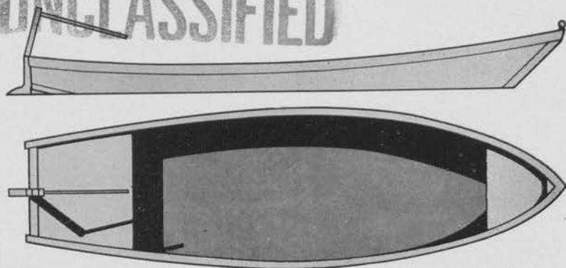
This craft, designated as a "float" or "tiller-type barge," is primarily used as a harbor lighter. Numerous variations of this type have been observed, including some up to 70' long and powered; others lashed together as a double or pontoon barge. Lack of armament and armor make this type extremely vulnerable.
