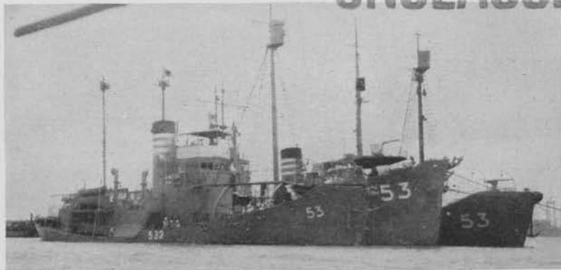
The two outboard vessels are KYO Class whale killers converted to serve as escort ships during the China campaign. Notice that the only apparent change from commercial appearance was the substitution of 3" guns for the forecastle harpoon. The ship in the center is a small engines-aft cargo type
