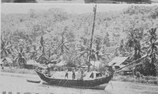
The craft illustrated on this page are typical N. E. I. sailing barges which carry on most of the inland-to-port river trade. Most are between 50' and 70' over all, are beamy, shallow-draft craft with a long spritsail. Steering is done by rudder or quarter paddles.
