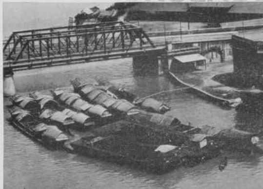
Large, wooden, rectangular scows like these are common to most Far-Eastern ports. They range up to 120' long and 300 tons in capacity; may be dumb or powered.
