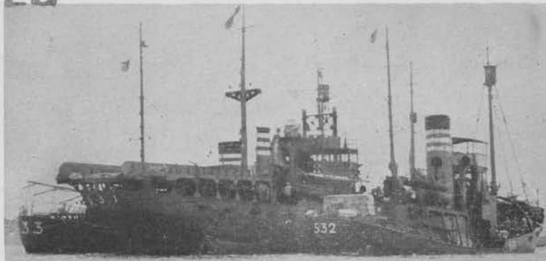
fitted with a stern ramp for transporting and launching harbor defense nets. Although little is known about these XAN (net tender) conversions, it can be assumed that this ship is typical. A complete list of all known XAN's is included in another section.
