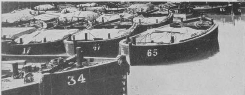
◀ A 70' cargo lighter with large-capacity open hold. Other photos on this page illustrate the junk-type of barge with its characteristic crude construction.
